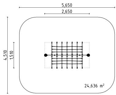
Lenght: 2 650 mm Width: 1510 mm Height: 1315 mm
