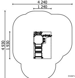
Lenght: 1 240 mm Width: 1 930 mm Height: 1 300 mm
