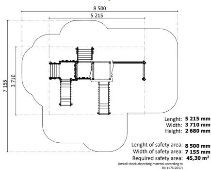
age 1,80 m height of fall 70 kg (heaviest part) 190 kg 2 h (without excavation and concreting)
